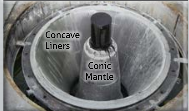
Complicated CWI Conical part with high pressure and abrasion in a rotary crusher
