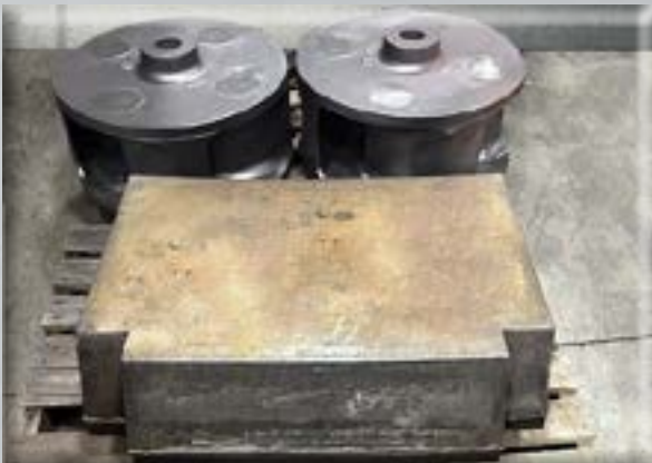
Bi-Metallic CWI liners for a SAG MILL Chute and rotors for pumps
