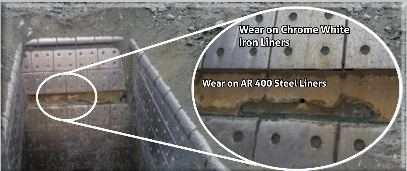
Wear comparison of inclined plan with severe impact and abrasion conditions in a hopper
