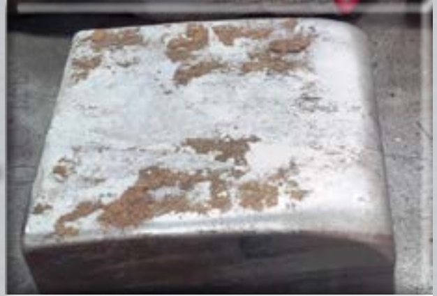
CWI HAMMER TIPS (+2.5X life vs standard parts that were protected by TUNGSTEN CARBIDE)
